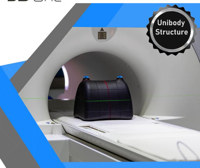
Large field MRI distortion phantom with embedded 3D grid for ease of alignment, with superior fluid filling / emptying facility
